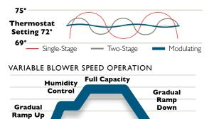
Gradual ramp up and down of the variable speed motor significantly reduce sound
